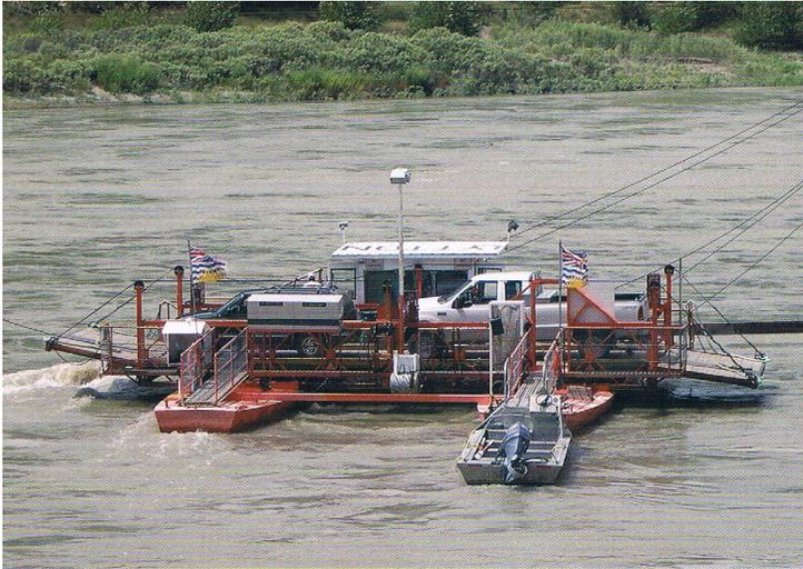
Just outside the town there is the Lytton Ferry that is operated, I believe, by the BC Ferry system. It is called a “reaction ferry,”\* that is, it is tied to a set of cables across the river that prevent it from running out of control down the river. The crossing is a free service. Fran and I did cross with the ferry just for the experience, but we left the RV parked on the highway side.
